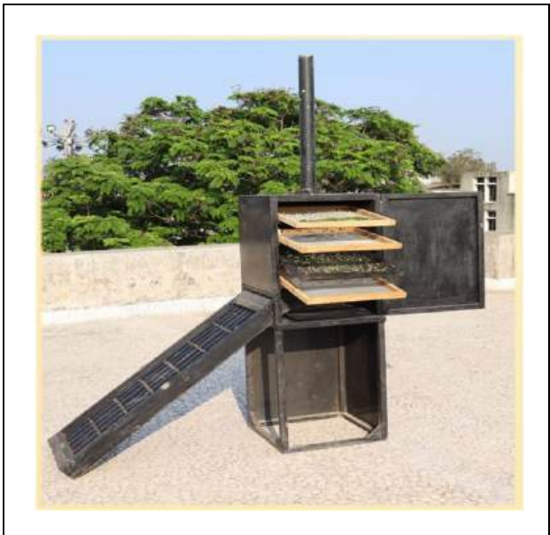
Figure.1: Low cost Solar dryer used in study showing drying products
